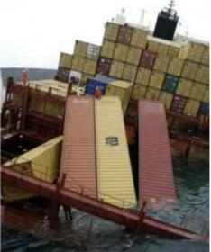
Bad ship design, flimsy containers, faulty twist locks, bad stowage, shoddy maintenance, poor seamanship, top heavy container stacks, mis-declared cargo, bad weather, commercial pressures, lack of compliance and communication failure all contribute to an increasing number of similar incidents.
