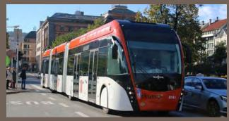
The buses are driven by an electric motor, with a battery charged by a biogas motor and by brake energy. The longest bus in Norway, 24 meters, and has special
