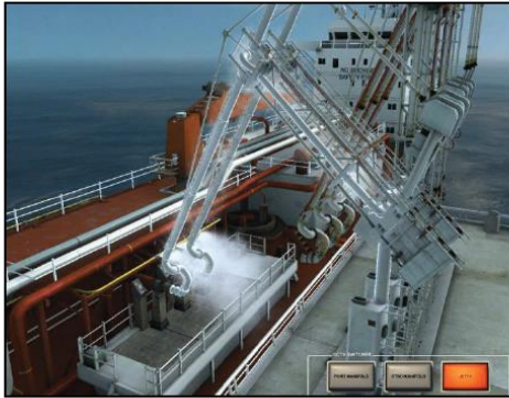
Manifold water spray
