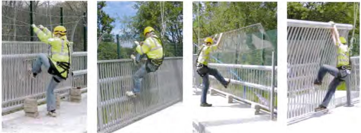
Figures 4a to 4d: Climbing trials on prototype extensions and replacements
