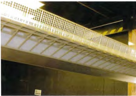
Figure 2: Sectional Model Wind Tunnel Testing of West Gate Public Safety Barriers
