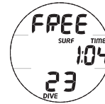
Fig. 30 - SURF MAIN (1 hr after dive 23)
