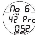
Fig. 38B - LOG 3 (Profile after 52 sec)
