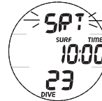
Fig. 64 - SRT ALARM (post dive)
