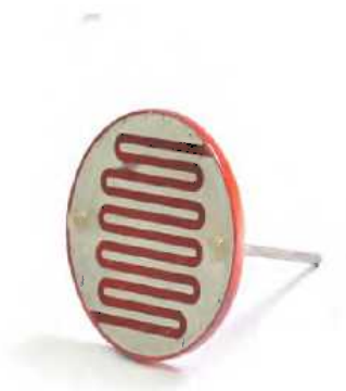
Lyssensor (light-dependent resistor - LDR), 3 mm diameter
