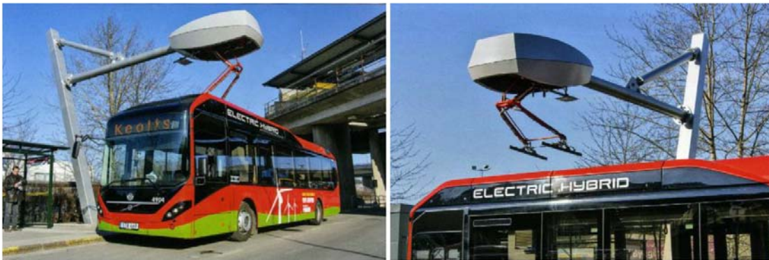
Figure 5 - example of opportunity charging from fixed point connecting to the bus
