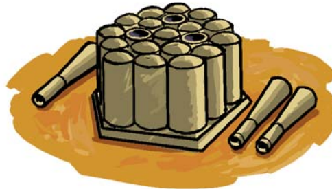
Figure 5. Illustrations of options for leaving the concrete substructure in situ, entirely with navigation lights (left) and cut down to the storage cells. Examples from Frigg cessation plan where the illustration to the left represents the approved solution for Frigg. Source: Total E&P Norge AS.
